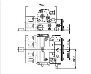
Version 4, 5 - valve fixed setting and inch valve mounted
