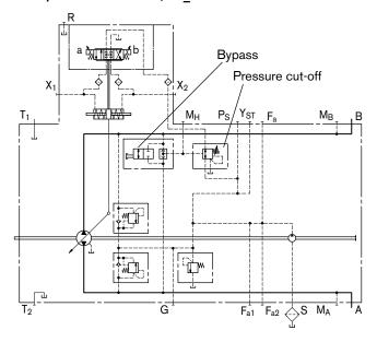
Schematic without pressure cut-off
