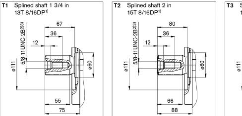
Before finalizing your design, request a binding installation drawing. Dimensions in mm.
