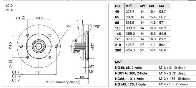
1) The through-drive flange is only supplied with the fastening thread corresponding to the ordering code designation.
