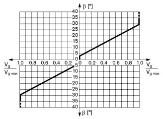
Swivel angle  $\beta$  at the control lever for pump displacement change:
