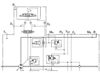
DA control valve fixed setting and braking inch valve mounted (4, 5) (only for pumps with DA control module)
