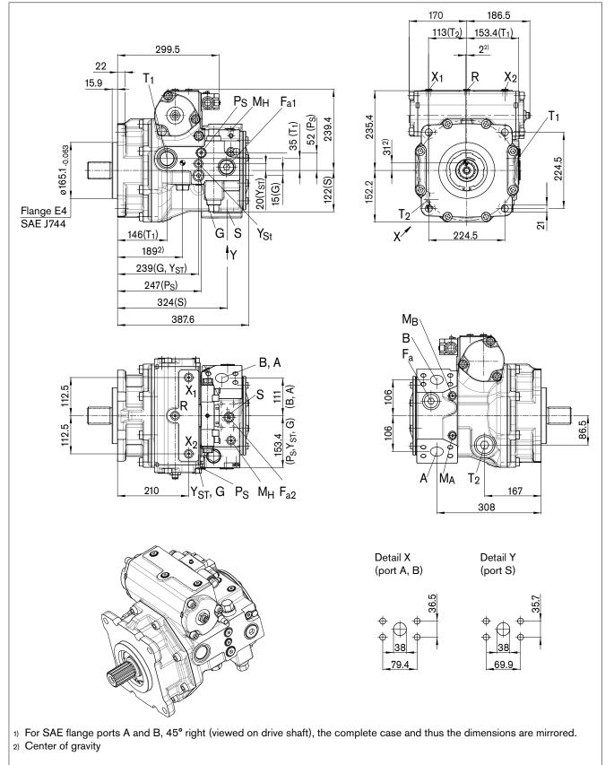
Before finalizing your design, request a binding installation drawing. Dimensions in mm.
