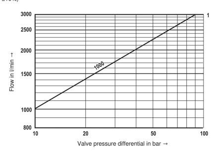
= Recommended flow limitation (flow velocity 30 m/s) in the valve connection bores
