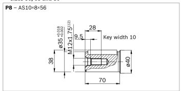
$_{\mbox{\scriptsize 1)}}$  Center bore according to DIN 332 (thread according to DIN 13)
