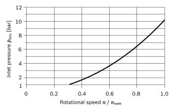
This diagram is only valid for the optimum viscosity range of  $v_{\text{opt}}$  = 36 to 16 mm<sup>2</sup>/s.
