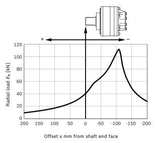
Maximum axial load  $F_{ax max}$  (with radial load  $F_{R}$  = 0):  $F_{ax max}$  = 49000 N  $\leftarrow$  +  $F_{ax max}$  = 35400 N  $\rightarrow$  -
