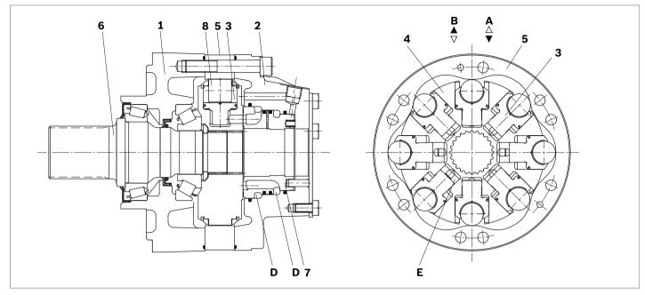
Hydraulic motors of the type MCR-A are radial piston motors incorporating a front case mounting and splined drive shaft. A-type motors are suitable for a variety of applications either as a direct drive into a gearbox or by fitting an external component (e.g. gear pinion or chain sprocket). They are suitable for use in open or closed circuit operations.
