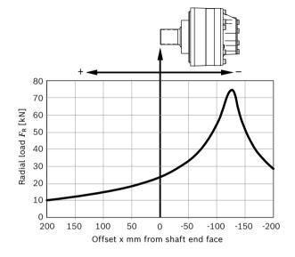
Maximum axial load  $F_{ax max}$  (with radial load  $F_{R} = 0$ ):  $F_{ax max} = 68000 \text{ N} \leftarrow +$  $F_{ax max} = 63400 \text{ N} \rightarrow -$
