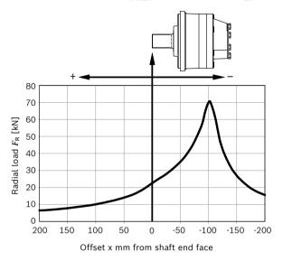
Maximum axial load  $F_{ax max}$  (with radial load  $F_{R} = 0$ ):  $F_{ax max} = 30700 \text{ N} \leftarrow +$  $F_{ax max} = 25200 \text{ N} \rightarrow -$
