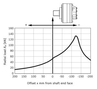
Maximum axial load  $F_{ax max}$  (with radial load  $F_{R}$  = 0):  $F_{ax max}$  = 95400 N  $\leftarrow$  +  $F_{ax max}$  = 82600 N  $\rightarrow$  - 10 **MCR-A** | Radial piston motor for frame integrated drives Dimensions
