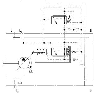
▼ Circuit diagram LA.DG with pressure cut-off, remotely operated
