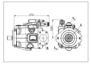
$_{\mbox{\scriptsize 1)}}$  ER7.: 191 mm when using a sandwich plate pressure reducing valve
