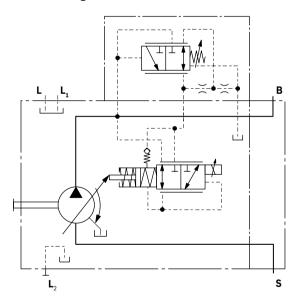
**1** The metering orifice (control block) and the line is not included in the delivery contents.
