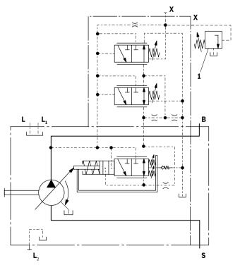
**1** The metering orifice (control block) and the line is not included in the delivery contents.
