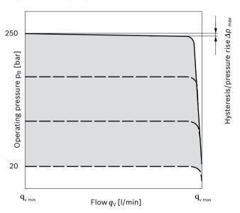
Characteristic curve valid at  $n_1$  = 1500 rpm and  $t_{fluid}$  = 50 °C.
