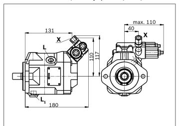
**▼** DRG - Pressure control, remotely operated (SAE)¹)
