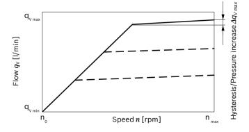
Characteristic curves valid for  $n_1$  = 1500 rpm and  $t_{fluid}$  = 50 °C.
