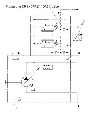
**1** The metering orifice (control block) and the line is not included in the delivery contents.
